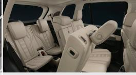
3<sup>rd</sup> row seats with 2<sup>nd</sup> row of seats incl. comfort entry and infinitely variable electric seat backrest tilt adjustment and fore-and aft adjustment incl. Comfort cushions.
